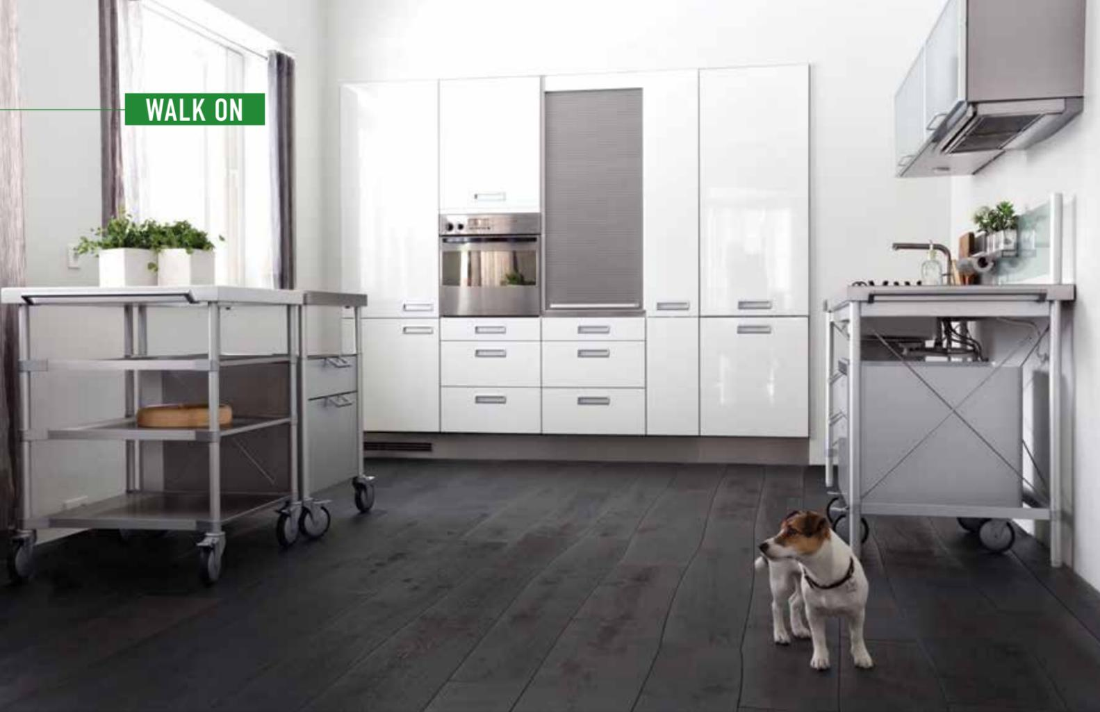
factory-finished wood flooring, which is pre-finished by the manufacturer. "Have it finished onsite if you want a smooth, flat floor," said Bradley. But if time is of the essence, go with the finished option, as you'll be able to walk on the flooring soon after the installation.
